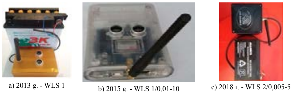
Figure 2 - Prototypes of water level sensors developed at KazSRIWE LLP in recent years
